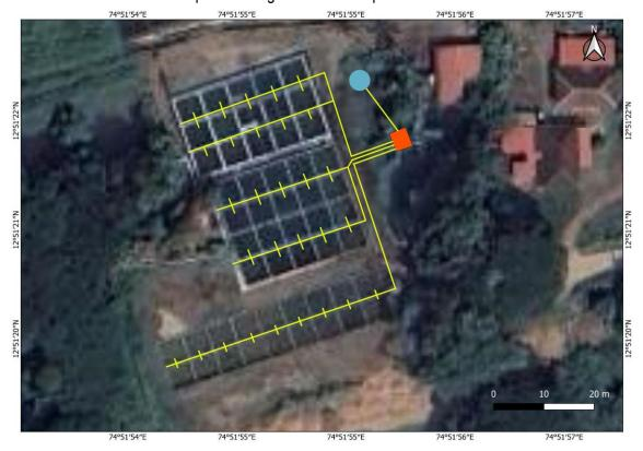
Schematic diagram location of ponds and tentative pipeline & water source point. (BLUE - circle: open well; RED rectangle - Pump shed, yellow lines: tentative pipeline across existing aquaculture ponds)
