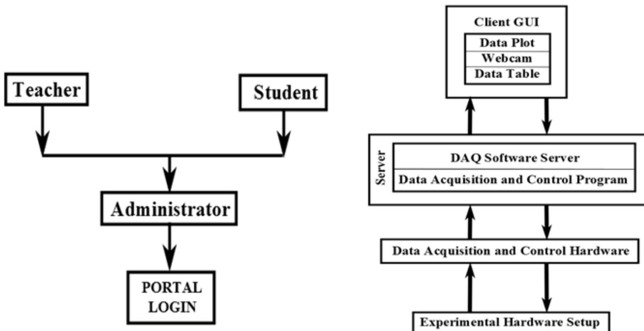
Figure 5. Flow chart explaining concept of Remote Triggered and Monitoring Second Order Ocean Wave profile Generator system setup
