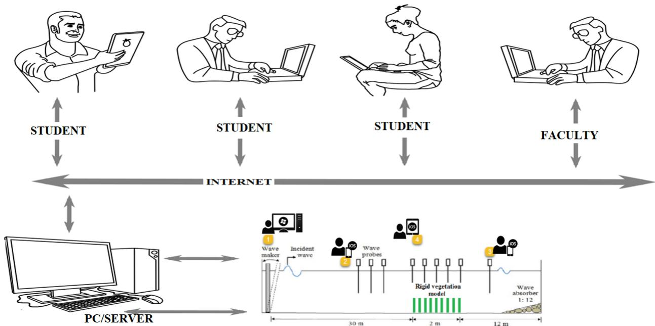
Figure 4. Schematics for concept of “Remote Triggered and Monitoring Second Order Ocean Wave profile Generator system”
