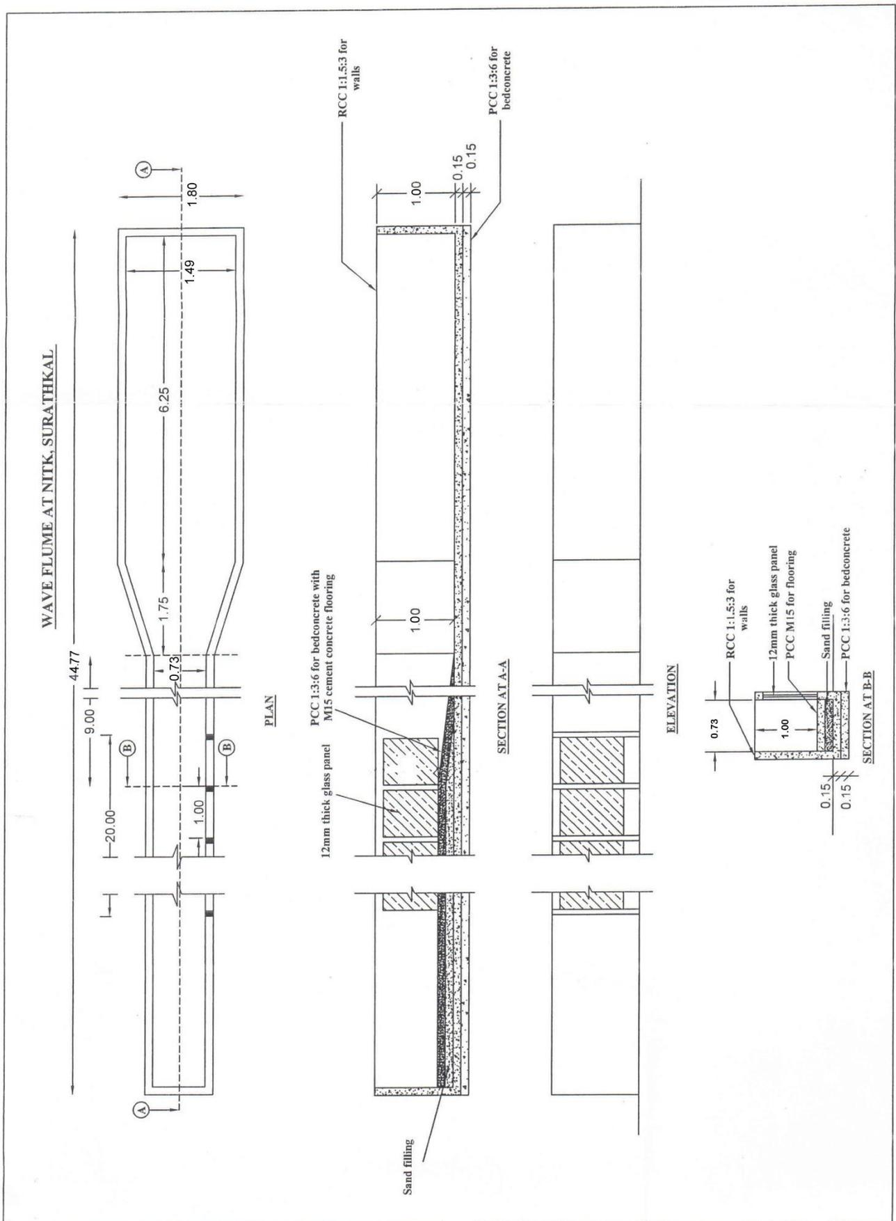
Figure 7. wave flume Dimensions
